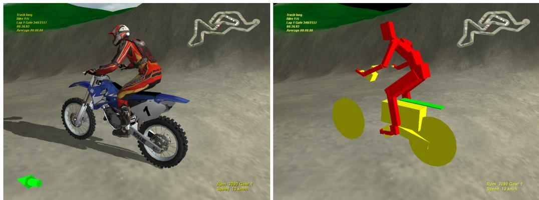
Figure 2.8: Bike Physics: The bike and biker as seen in the game and their associated collision and dynamic objects used in the simulation.
