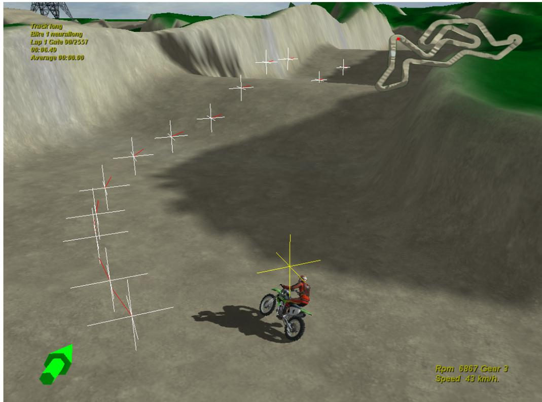
Figure 4.1: Inputs of the AI: positions of the centre of the track, used as inputs to the ANN.
